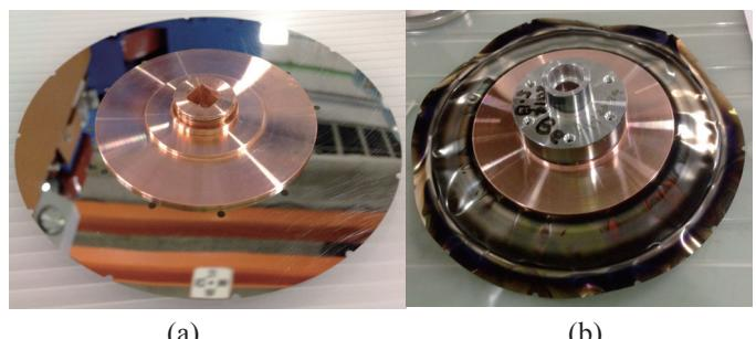
Fig. 2. (a) New specially designed Be disk and (b) after irradiation. Deformation was moderated.
