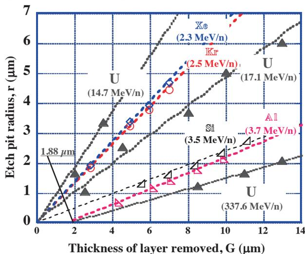
Fig. 1. Etch pit growth curves for U ions (14.7, 17.1 and 337.6 MeV/n), Xe ions (2.3 MeV/n), Kr ions (2.5 MeV/n), Si ions (3.5 MeV/n), and Al ions (3.7 MeV/n). Each energy for other indicating ions is close to that of the Bragg peaks.
