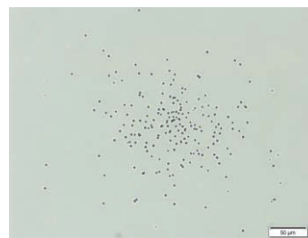
Fig.2. Profile of the extracted beam, when the distance between the exit of the capillary and the CR-39 was 2 mm. The scale corresponds to 50 \mu\text{m} .
