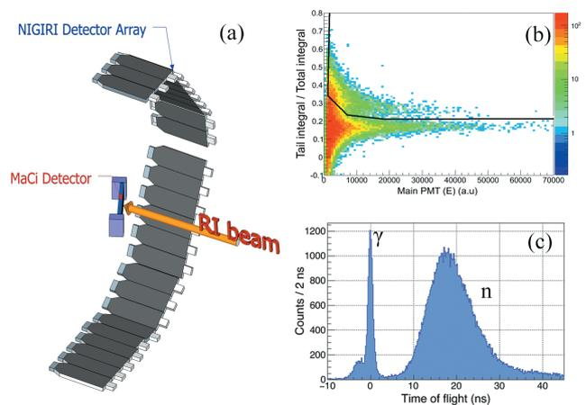
Fig. 1. A schematic view of the experimental setup employing the NiGIRI and MaCi detectors (a).  $^{252}\text{Cf}$  source test: PSD versus total integral. PSD cut (black lines) has been applied to select neutron events (b). The time-of-flight spectrum from all NiGIRI detectors after applying PSD cut (c) (small tail prior to gamma ray peak appeared due to backscattering).
