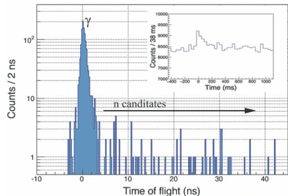
Fig. 2. Combined neutron time-of-flight spectrum associated with the implantation of the RI beam in the MaCi detector. The inserted figure shows the time correlation between decay events and implantation events from the MaCi detector.
