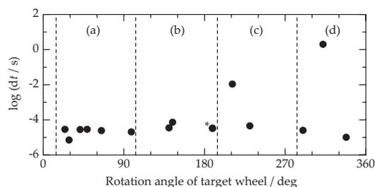
Fig. 1. Decay time of SF events in  $^{208}\text{Pb} + ^{48}\text{Ti}$  reaction at  $E_{\text{lab}} = 242 \text{ MeV}$ . The abscissa shows a rotation angle from a specific position. Regions of (a) to (d) correspond to the excitation energies, (a)  $E^* = 22.2 \text{ MeV}$ , (b) 26.3 MeV, (c) 29.5 MeV, and (d) 17.8 MeV. \*Two symbols almost overlapped.
