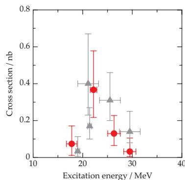
Fig. 2. Excitation functions of  $^{254}\text{Rf}$  production in  $^{208}\text{Pb} + ^{48}\text{Ti}$  reaction. Circles and triangles show results of this work and reference,<sup>3)</sup> respectively.
