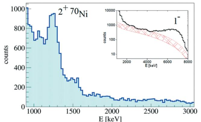
Fig. 1.  $2^+ \rightarrow 0^+_{\text{gs}}$  E2 transition in  $^{70}\text{Ni}$ . In the inset, high-energy  $\gamma$  ray spectra are shown till 8 MeV. The shaded area is the contribution from the thick gold target, deduced from the measured spectra at backward angles and the projectile GDR-tail calculated with a statistical model.
