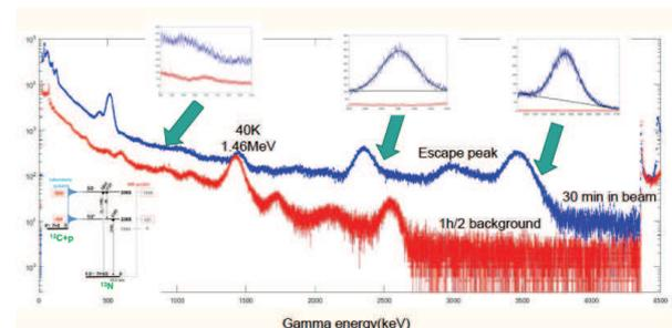
Fig. 2. An example of the  $\gamma$ -ray spectra. The histogram in blue color was obtained in the "in-beam" measurement for the  $^{12}\text{C}(p,\gamma)^{13}\text{N}$  reaction with a 2 MeV proton beam. Two  $\gamma$  ray peaks corresponding to the two low-lying resonances in  $^{13}\text{N}$  (see the inset for the level diagram) are clearly seen. The other peaks are of the natural background, which is identified in the spectrum taken without the beam (in red color).
