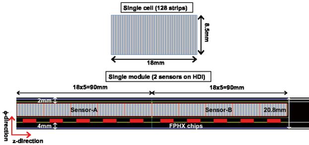
Fig. 1. The drawings of an L0 single cell and a module consisting of ten cells on HDI.
