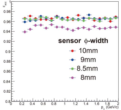
Fig. 2. The simulated L0 acceptance with different  $\phi$ -widths.
