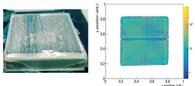
Fig. 1. (Left) Segmented YSO scintillator before coupling to the photomultiplier. (Right) Implantation profile recorded by the segmented YSO detector.
