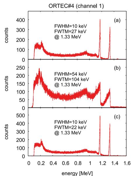
Fig. 2. Example of <sup>60</sup>Co spectrum: (a) before MT, (b) after MT, (c) after annealing process.
