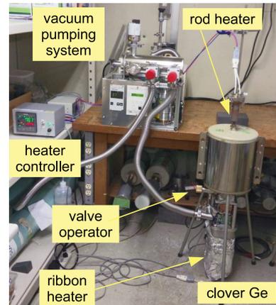
Fig. 1. The pumping and annealing system.
