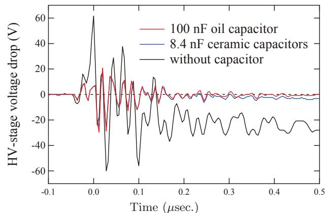
Fig. 2. Voltage drop of the H.V. stage in a short time range around the switching noise of the grid pulse.
