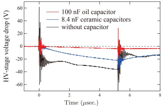
Fig. 1. Voltage drop of the H.V. stage of the electron gun in the time range of the grid pulse of 5  $\mu$ s.
