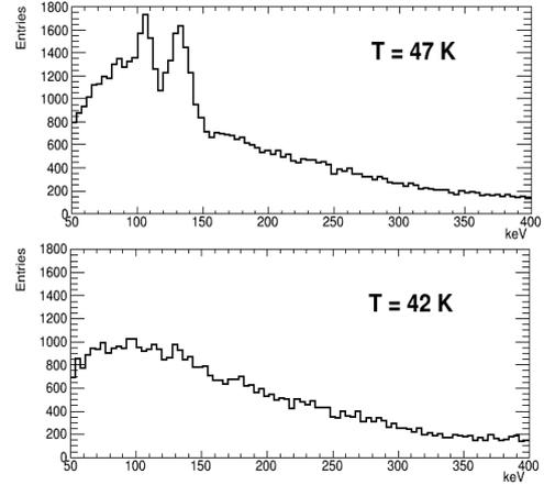
Fig. 2. Upper panel, shows the delayed nitrogen X-rays lines at a temperature of 47 K. In the lower panel the same spectrum is shown at a temperature of 42 K.
