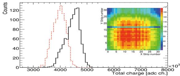
Fig. 1. Total charge detected by the hodoscope before (red dashed line) and after (black solid line) the tuning of the magnets and, in the insert, the two dimensional beam profile of 1 mm per strip.
