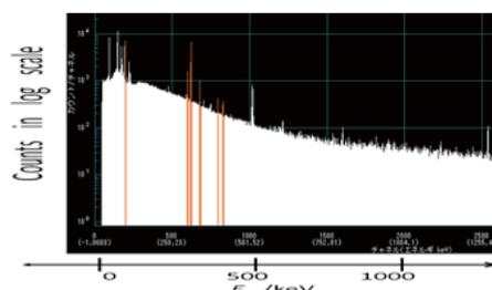
Fig. 2. An example of  $\gamma$  spectrum of isolated Np solution sample. Colored regions correspond to the most prominent emission of U-X ray and  $\gamma$  emissions from Pa-233.
