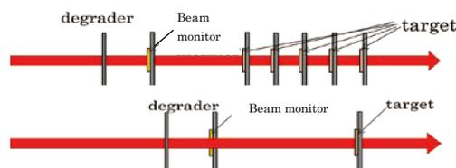
Fig. 1. Schematic illustration of target stacks for the reaction of  $^{232}\text{Th}$  with  $^7\text{Li}$  ions.
