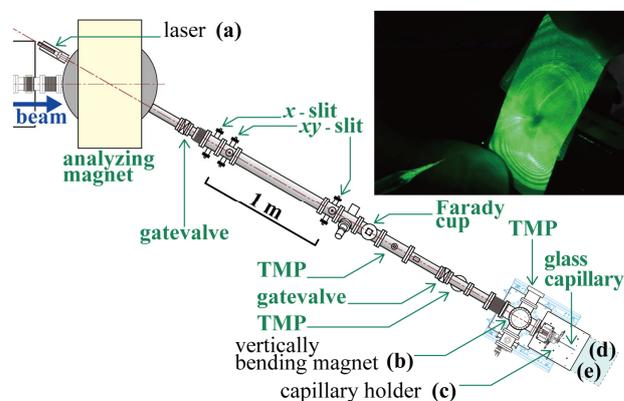
Fig. 1. The beam line of the new microbeam system. The symbols (a)–(e) are explained in the text. The degree of vacuum level is kept better than  $10^{-5}$  Pa.
