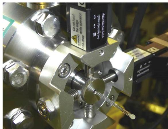
Fig. 2. Capillary holder with a remote tilt system controlled through Ethernet. The glass tube will be replaced with a tapered glass capillary optics to produce microbeams.
