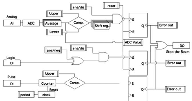
Fig. 1. Logic diagram of upgraded fast interlock system.
