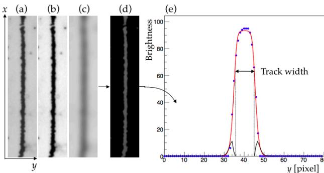
Fig. 1. Image processing method to obtain track width.
