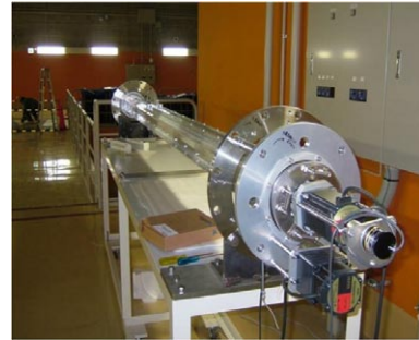
Fig. 1. Field-mapping device (before installation inside the STQ)
