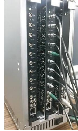
Fig. 2. DSP system consisting of two 9-ch ADCs and our daughter modules (TechnoAP, APU7110-A40).
