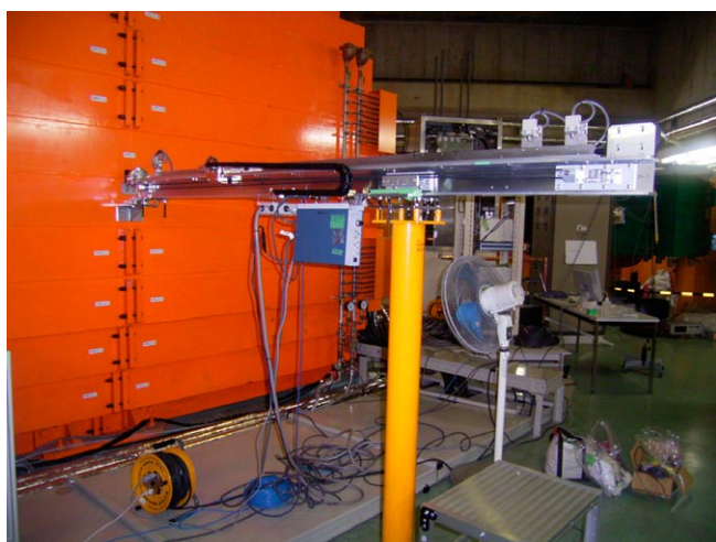
Fig. 1. Photograph of the magnetic field measuring system. The left of figure is a backside of the magnet yoke.
