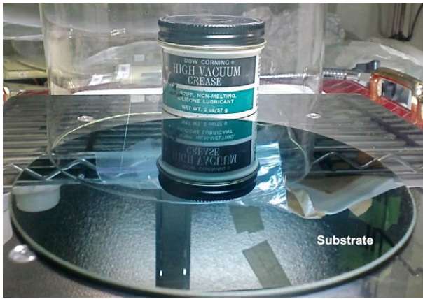
Fig.4. The glass substrate on which evaporated carbon was deposited.
