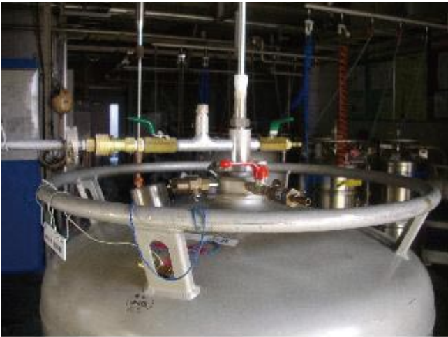
Fig. 4. The container is connected to the recovery line using the newly developed cryogenic coupler.
