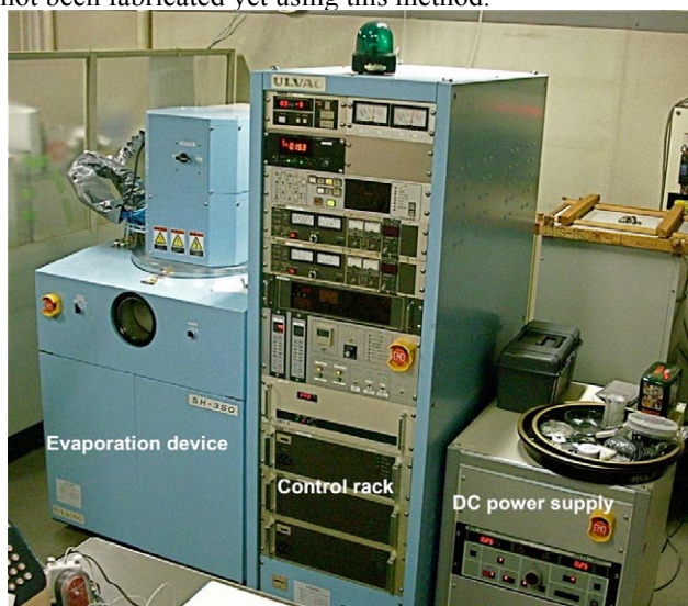
Fig.1. High-vacuum evaporation system (SH-350 by ULVAC).
