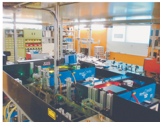
Fig. 1. The photograph of new PALIS lasers: shining two dye lasers pumped by YAG laser.
