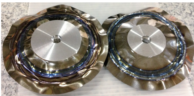
Fig. 1. Polished Be disks after irradiation (Right: Disk 2, Left: Disk 3).
