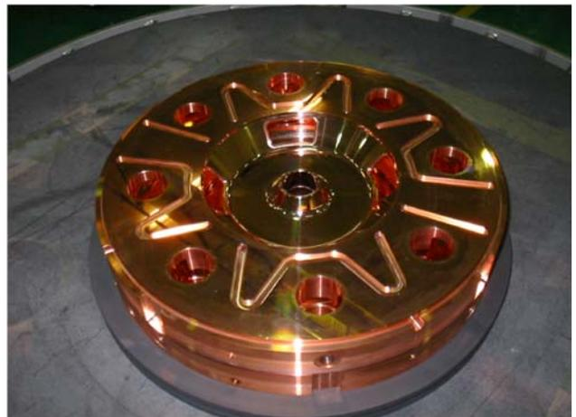
Figure 11: A half cell of the J-PARC ACS. The view is from the accelerating cavity side.
