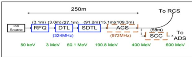
Figure 6: Scheme of J-PARC linac.
