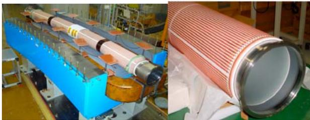
Figure 15: Ceramics chambers used for the J-PARC RCS. The left is for the bending magnet, while the right for the quadrupole magnets.
