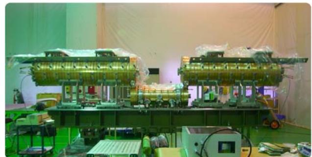
Figure 12: Lowest energy ACS module that was already powered.
