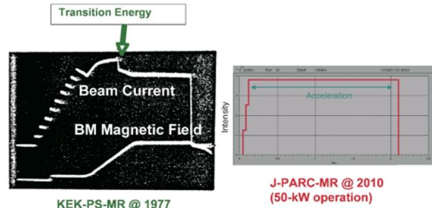
Figure 13: Beam current variation patterns during the injection and the energy ramping. The left is that of the KEK-PS MR (courtesy of KEK Archives Office), while the right is that of J-PARC MR. The original data points of the right figure were too thin to see. So, the data points were traced in a thick curve.
