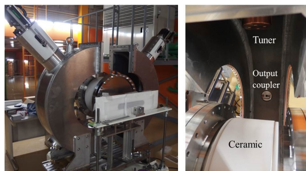
Figure 1: (Left): The resonant Schottky pick-up divided in half. The Schottky pick-up has a pillbox-type resonant cavity. (Right): Inside of the resonant cavity. In the upper part, a tuner for fine tuning the resonance frequency is shown. In the lower part, a pick-up loop for detecting the induced magnetic flux is shown.
