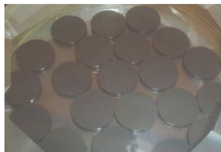
Figure 3: Photograph of 1-mm uranium-oxide-coated target disks. These disks are 20 mm in a diameter and 1 mm in a thickness.
