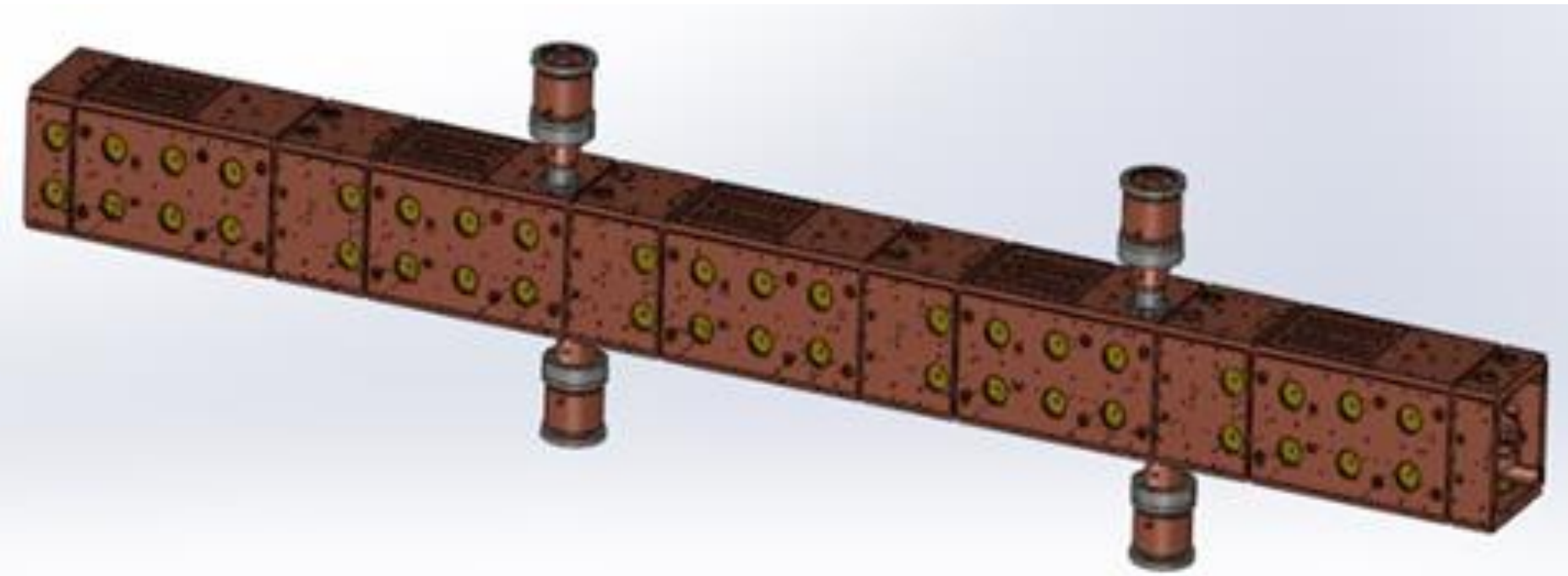
Figure 1: 3D model of the deuteron beam RFQ.
