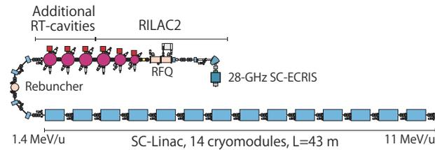
Fig. 1. Layout plan of new linac injector.
