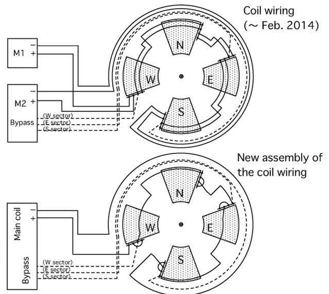
Fig. 1. Wiring of the RRC main coil.
