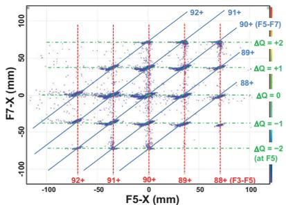
Fig. 1. Spectrum of F7- $x$  vs. F5- $x$  measured with a  $^{238}\text{U}$  primary beam after it passes through PPACs at F3. Red and blue lines have information on the F3-F5 dispersion and the F5-F7 magnification, respectively. The F3-F7 dispersion and the F5-F7 dispersion can be deduced from green lines.
