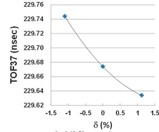
Fig. 2. Measurement of  $(\ell|\delta)$  with primary beams. TOF from F3 to F7 was measured for each charge state by selecting the charge state with the F5 slits. The solid curve represents a quadratic fitting, and the slope corresponds to  $(\ell|\delta)$ .
