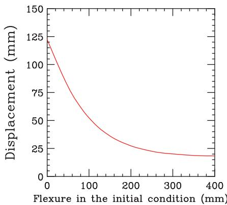
Fig. 1. The flexure dependence of Kevlar textile displacement.
