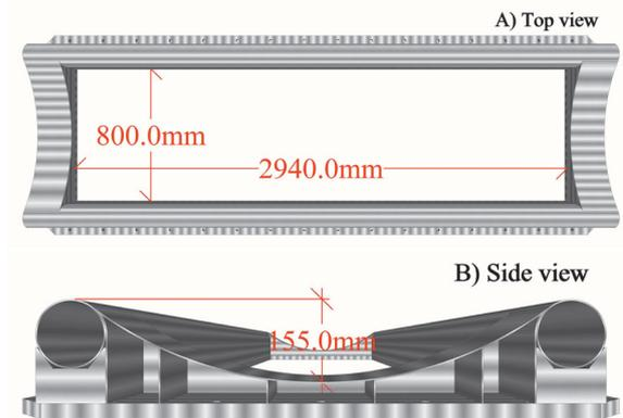
Fig. 2. Drawing of the full-size partition window.
