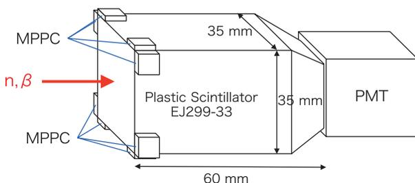
Fig. 1. The overview of the prototype NiGIRI detector.
