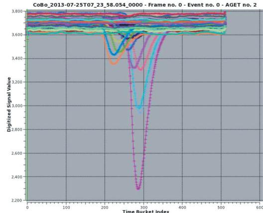
Fig. 1. Cosmic signal detected by S $\pi$ RIT-TPC with GET electronics. Each line corresponds to one channel. One AsAd board contains four ASIC chips (AGET). One ASIC corresponds to 32 channels. The GET system employs SCA type flash ADC. Up to 512 time buckets can be used for analog data buffering. The pedestal is not suppressed in this figure.
