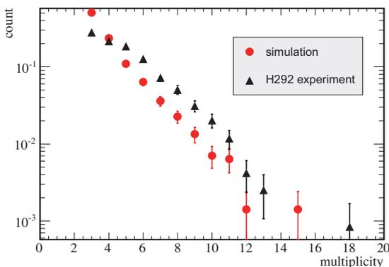
Fig. 1. Comparison of charged-particle multiplicity distribution between the simulation and the H292 experiment, with multiplicities of more than 2. The simulated distribution is normalized to the experimental yield.
