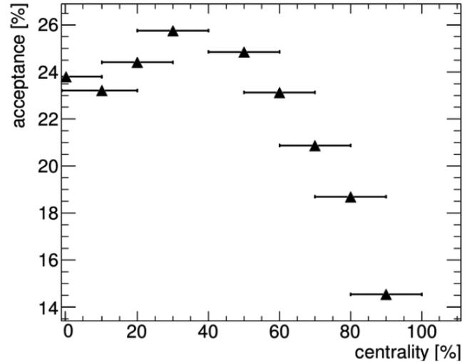
Fig. 2. Acceptance of the trigger scintillator array as a function of the centrality in 300 AMeV  $^{124}\text{Sn} + ^{124}\text{Sn}$  collisions when the trigger scintillator arrays were installed to cover the polar angles ranges of  $-40 < \theta < -20$  and  $20 < \theta < 40$  degrees.
