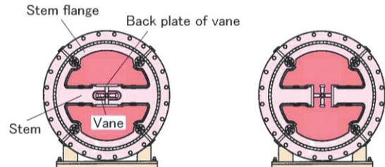
Fig. 2. Cross-sectional views of INS-type SCRFFQ (left) and modified RFQ (right).
