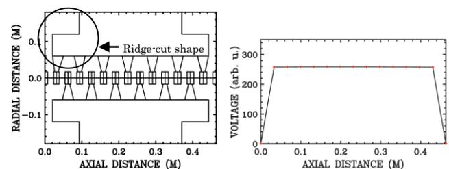
Fig. 3. Longitudinal sectional view (left) and gap-voltage distribution (right) for the 158.1-MHz IH tank1.
