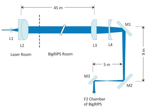
Fig. 1. Planned optics system for transportation of laser beams to PALIS.
