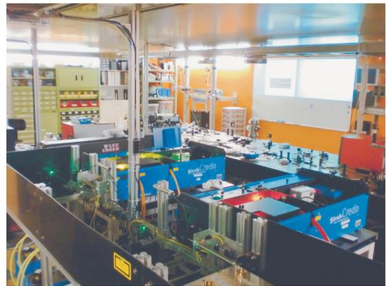
Fig. 1. The photograph of new PALIS lasers: shining two dye lasers pumped by YAG laser.
