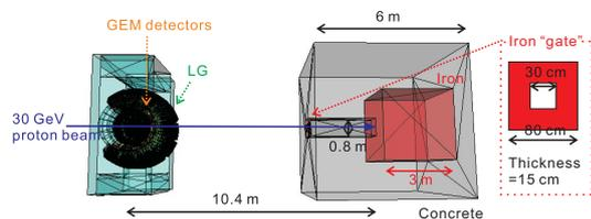
Fig. 1. Schematic model of the E16 experiment used in the simulation. The area is surrounded by concrete blocks, and is filled by air.
