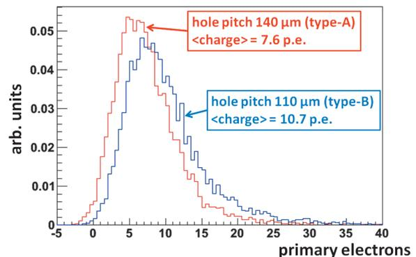
Fig. 2. Charge distribution of two different photocathodes.
