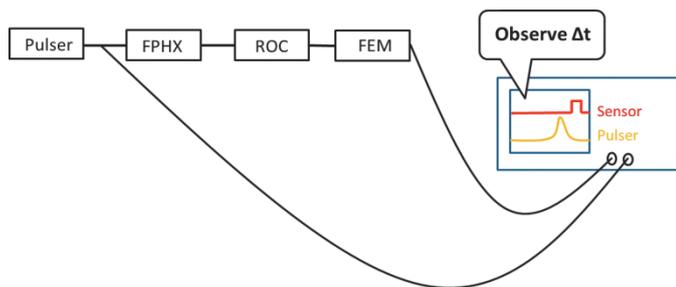
Fig.1 Setup of the timing measurement using a scope and FVTX readout devices<sup>1)</sup>
