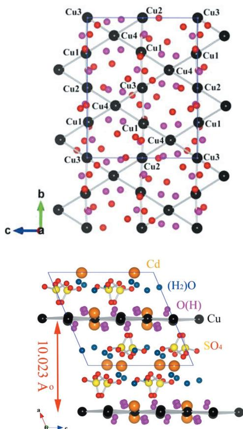
Fig. 1. Structure of  $\text{Cd}_2\text{Cu}_3(\text{OH})_6(\text{SO}_4)_2 \cdot 4\text{H}_2\text{O}$ .
