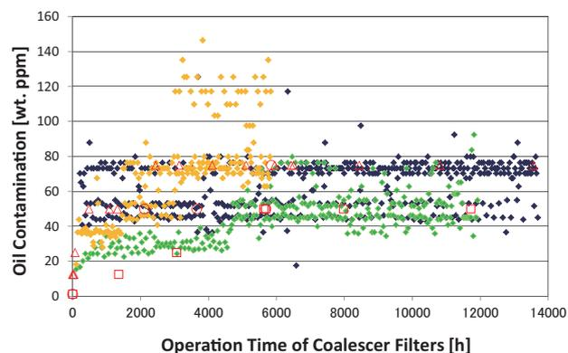
Fig. 1. Oil contamination at the entrance of the second coalescer vessel (3SP).
