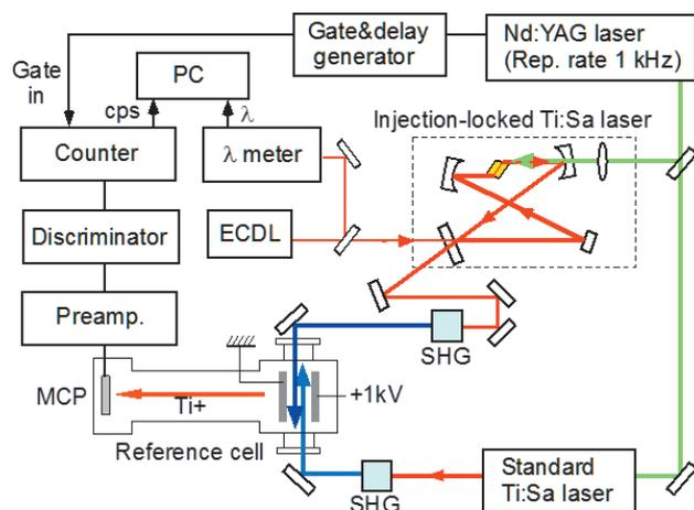
Fig.1 Experimental setup for HR-RIS on Ti
