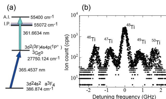
Fig.2 (a) Ionization scheme on Ti
