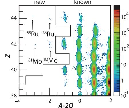
Fig. 2  $Z$  versus  $A-2Q$  particle identification plot for projectile fragments produced in the reaction  $^{124}\text{Xe}+\text{Be}$  at 345 MeV/nucleon.
