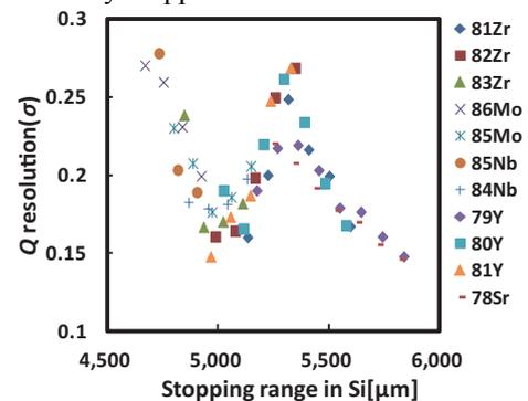
Fig. 1 Charge state ( $Q$ ) resolution as a function of the stopping range
