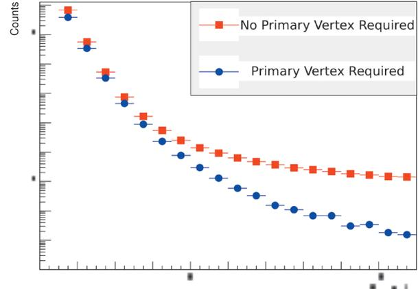
Fig. 2. Uncorrected hadron  $p_T$  spectra for different purity cuts. At high  $p_T$ , the spectrum without the DCA requirement appears unphysically flat while the spectrum with the DCA requirement continues to fall.
