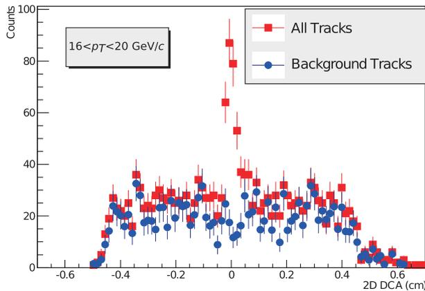
Fig. 1. Raw DCA distribution in the transverse plane. The peak around zero DCA is dominated by real tracks. The underlying background comes from random tracks and weak decays. The fall-off at  $\pm 0.4$  cm is an artifact of the tracking algorithm.
