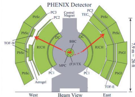
Fig. 2. Cross section of the PHENIX detector. The relative position of VTX west/east and DC west/east can be moved during the experiment.
