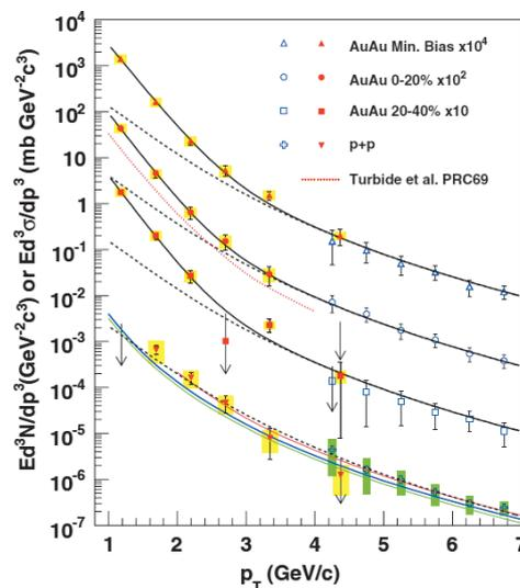
**Figure 3** Invariant cross section (p+p) and invariant yield (Au+Au) of direct photons as function of  $p_T$ . Published in Phys. Rev. Lett. 104, 132301 (2010).
