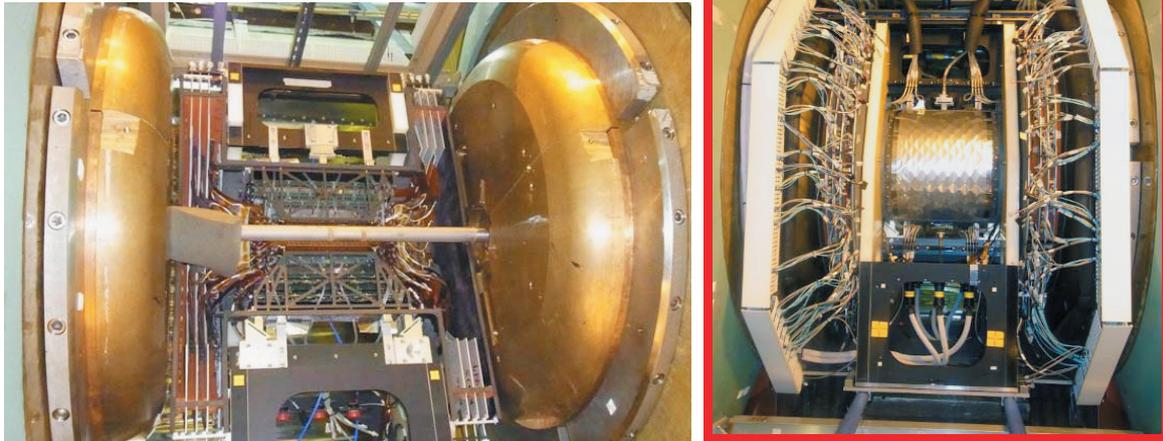
**Figure 4** Left: a picture of West half of VTX detector installed in PHENIX experiment. The interior of the detector can be seen. Right: The VTX detector completed with all cables, cooling tubes and dry gas connections.
