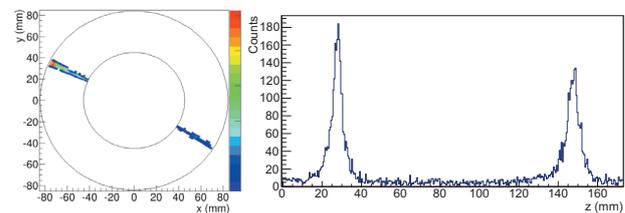
Fig. 2. (Left) Two-proton-like event. (Right) Reconstructed vertex position in the beam direction for a  $^{20}\text{Ne}$  beam at 350 MeV/u and two 0.5 mm thick  $\text{CH}_2$  targets separated by 124 mm.
