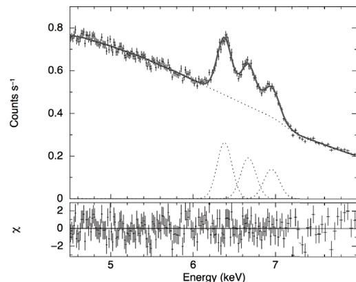
Fig. 1. Time-average X-ray CCD spectrum of V1223 Sgr. Thermal bremsstrahlung continuum and three atomic emission lines from neutral Fe (6.4 keV) and highly ionized Fe ions (6.7 and 6.9 keV).
