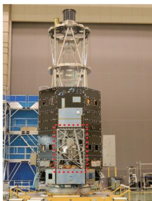
Fig. 1. Flight model of the *ASTRO-H* satellite body in a vibration test, including the engineering model of the SXS dewar<sup>2)</sup> on the inside. The red dotted square shows a window at the satellite panel, through which the harnesses are exposed to the space and MMODs can enter.
