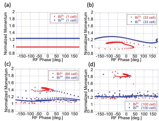
Fig. 2. Result of longitudinal phase space distribution. Red:  $\text{Bi}^{2+}$ , Blue:  $\text{Bi}^{3+}$ . The ordinate axis shows momentum normalized to  $\text{Bi}^{2+}$  initial momentum. The abscissa shows RF phase. (a) Initial distribution, (b) after pre-bunching, (c) after capturing  $\text{Bi}^{2+}$ , (d) after acceleration.
