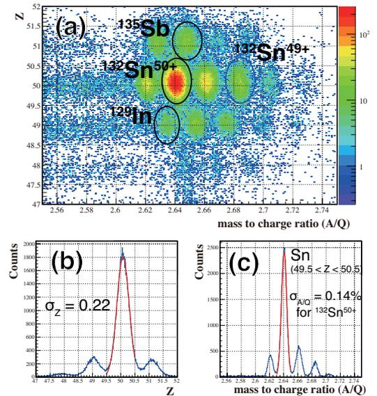
Fig. 1. (a) A SAMURAI PID spectrum with respect to  $Z$  and  $A/Q$  for non-reacted events with empty target cell. (b)  $Z$  distribution for all beam component and (c)  $A/Q$  distribution for Sn isotopes. The resolution of  $Z$  and  $A/Q$  are  $\sigma_Z = 0.22$  and  $\sigma_{A/Q} = 0.14\%$  for  $^{132}\text{Sn}^{50+}$ , respectively.
