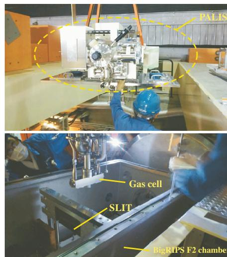
Fig. 1. The upper photo shows the entire PALIS integrated with the F2 chamber's roof. The lower photo is the gas cell part in PALIS.
