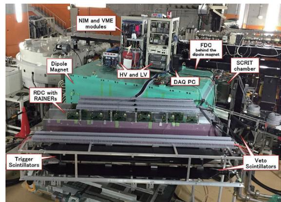
Fig. 2. Appearance of WiSES setup at SCRIT experiment.
